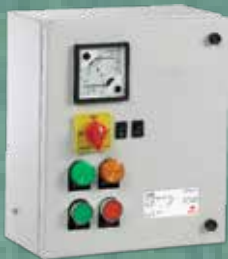
3 \phi DOL Starter Submersible Pump Controller Ratings - 0.75 kW to 11 kW (1 HP to 15 HP)
